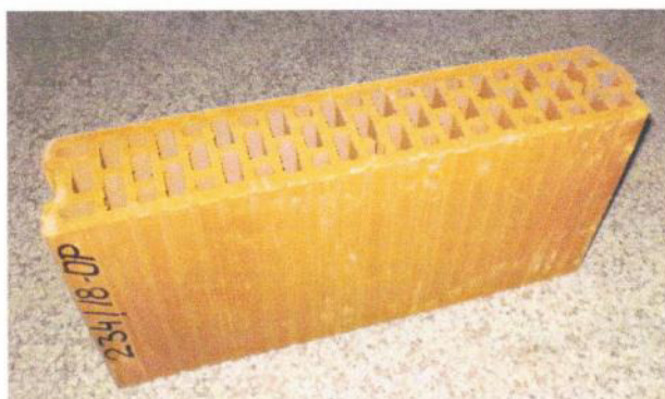
šuplji blok SRPS B.D1.015:2002-povučen / V - 500x100x238 – 150 - I
